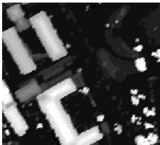
Fig.3. The LIDAR derived DSM imagery.
