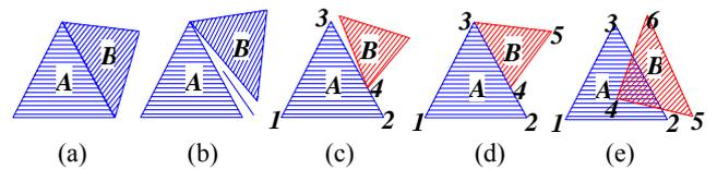
Figure 4. Regular togetherness of triangles (a), (b) and the irregular togetherness of triangles (c), (d), (e)
