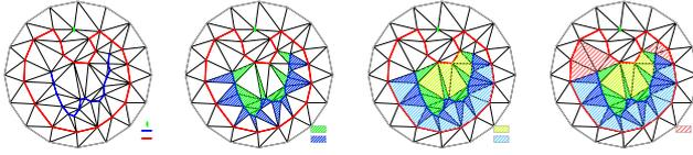
(a)  $\mathcal{CDT}$  building on node structure, vector chain structure and directed cycle structure (b) Direct taking out the left and right side of vector chain structure (c) Taken left and right side of chain by the including & approximating theorem (d) Triangles associating with start and end node of chain
