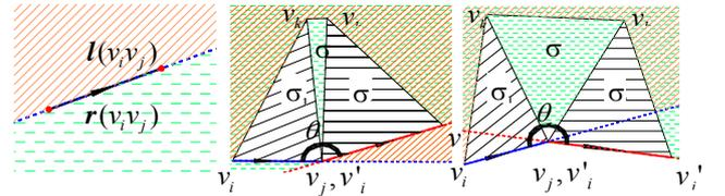
(a) Left and right semi-plane of chain (b)  $0 < \theta < \pi$  (c)  $\pi < \theta < 2\pi$
