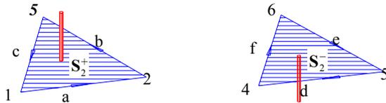
(a) Positive vector product and vertices of triangulation anticlockwise ordering (b) Negative vector product and vertices of triangulation clockwise ordering
