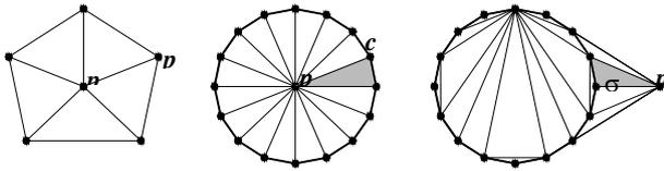
Figure 1. (a) Points and adjacency relationships between them in a TIN. (b) One point and one polygon in a CDT, the point  $p$  locates in the  $c$ 's interior. (c) One point and one polygon in a CDT, the point  $p$  locates in the  $c$ 's exterior.
