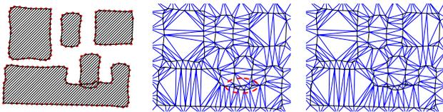
(a) Constrained chain set  $C$  and node set  $P$  (b)  $\mathcal{D}(P)$  (c)  $\mathcal{CD}(P)$
