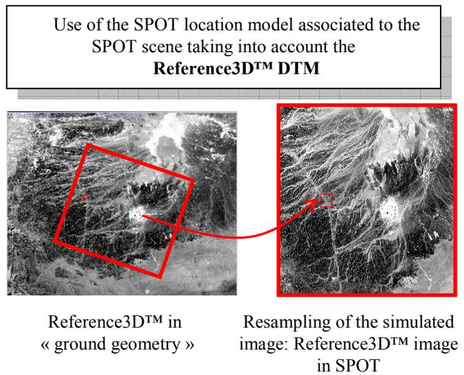
Figure 2 . Resampling of Reference3D™ tiles into “raw sensor geometry”
