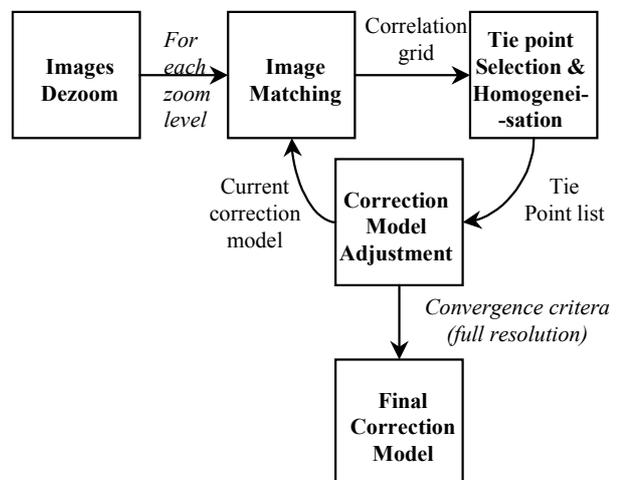
Figure 4. Correction model estimation by multiresolution image matching
