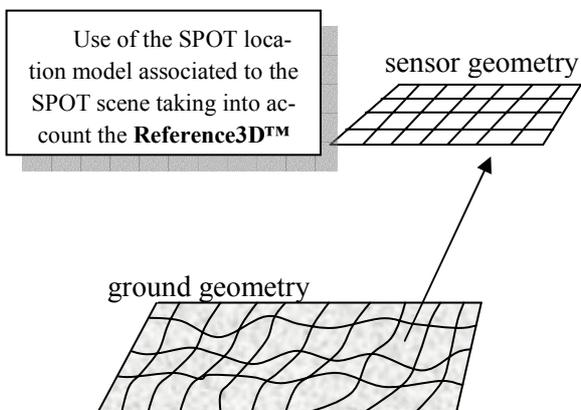
Figure 3. Computing simulated image resampling grid
