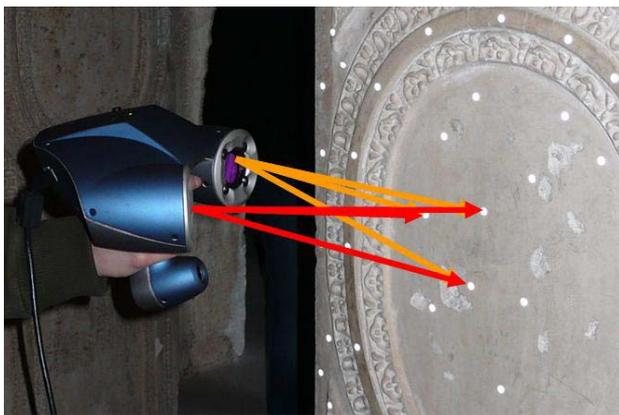
Figure 2. The system is based on association of two crossed laser liner cameras and a laser plotter
