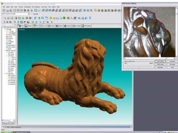
Figure 12. Texture mapping of the model
