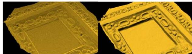
Figure 4. Triangular mesh surface created in real time during the acquisition phase
