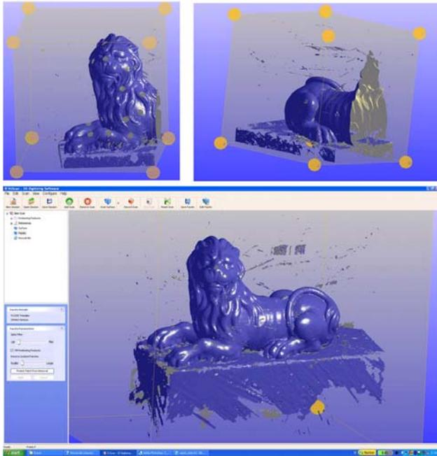
Figure 7. Both lions were acquired in two boxes of 200 x 200 x 200mm with the basic unit of voxel of 0.39mm. The dimension of each lion is around 171 x 138 x 269mm
