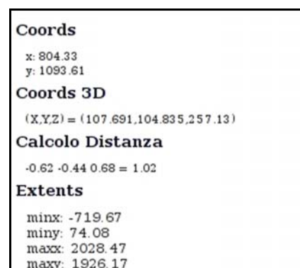
Figure 10. Distance measurement output in the info section (B Figure 3). X, Y, Z and 3D distance in meters (from left to right) The design of this tool and of the subsequent analysis ones was based on AJAX technology, which makes it possible to avoid
