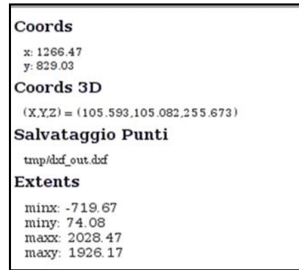
Figure 11. DXF export tool: after the selection phase ends, the DXF is created in a web accessible location, and the link for its download appears in the info section.
