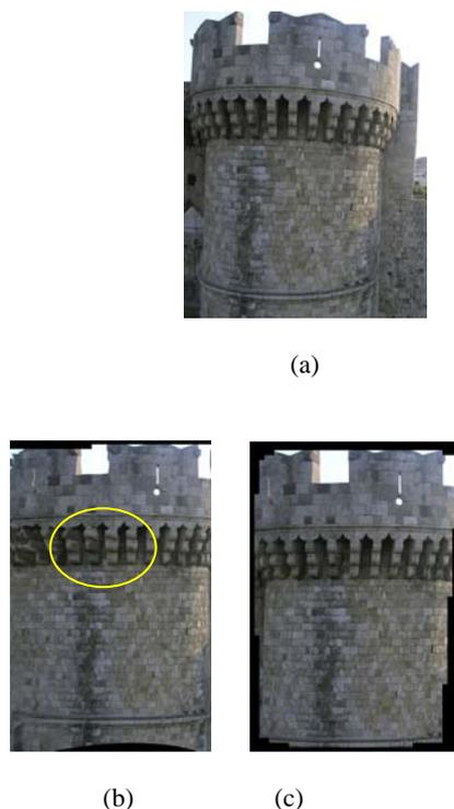
Figure 4: (a) Image of right tower (complex geometry) and orthophoto (b) with DSM and (c) with edited DSM
