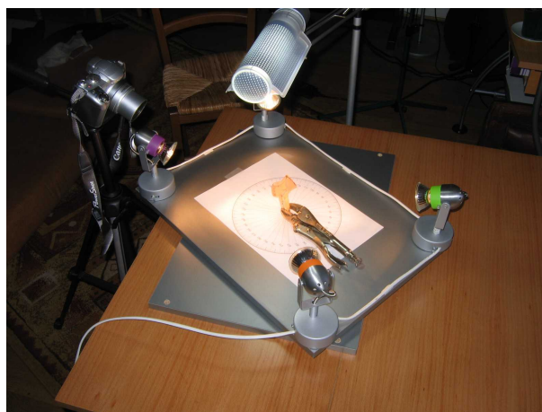
Figure 1: The device used for image acquisition. On the left, the camera on its tripod
