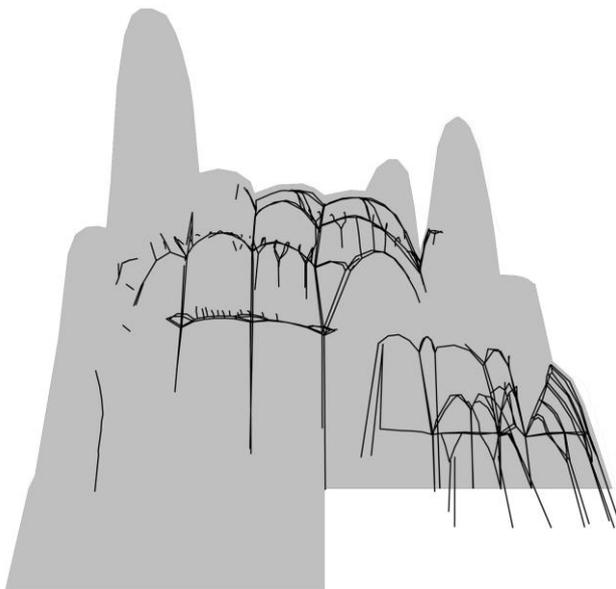
Fig. 6. Side view - results of multi-image photogrammetry
