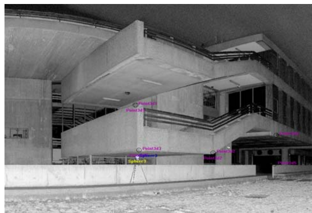
Figure 9. Registration using spherical targets in FARO Scene
