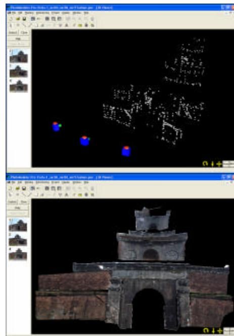
The second method has instead been used for the other monuments. In this sense the system of speditive photogrammetry has proved itself specially useful as it is based on some certain measures and on digital photographs taken in the appropriate way.
