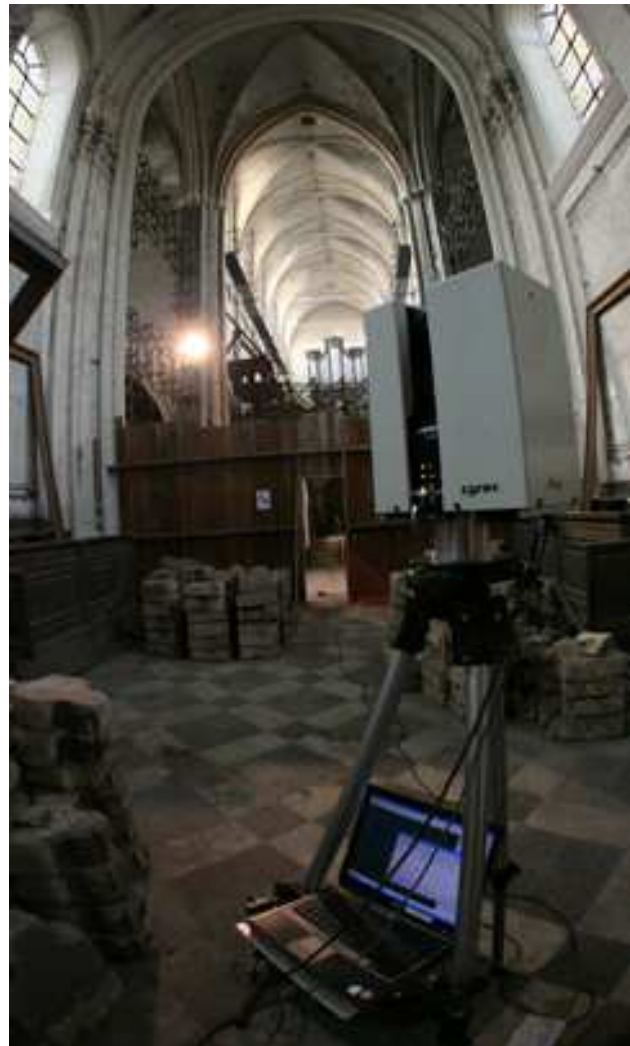
Figure 4: inside St.-James church in Leuven, scanning using a phased-base scanner provided by Plowman Craven and Associates, author.
