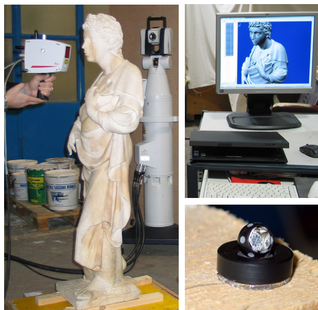
Figure 1: The Prophet survey, using a combined application of tracker system (left, on the back) and a hand laser scanner (left, front); data during acquisition phase are immediately aligned and referenced (right, top) thanks to mirror reflectors measured from both tracker positions.
