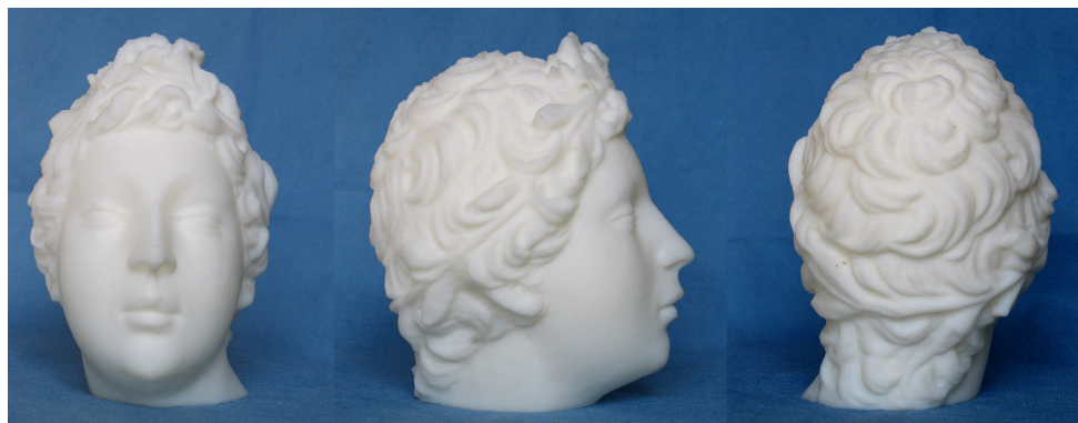
Figure 7: The solid model of the head, made in ABS by a FDM printer (working scheme on the left, see 4.2.1)
