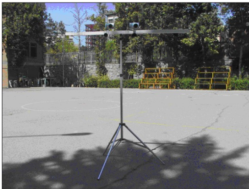
Figure 4. The stereo bar used for image acquisition
