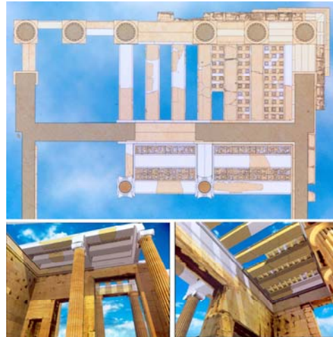
Figure 1. Proposed restoration of the ceilings. View from below (above), in the west hall (below left) and in the east portico (below right).
