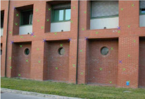
Figure 6: The calibration field; green markers used for image measurements, blue markers for topographic measurements, b/w targets for both kind of observations
