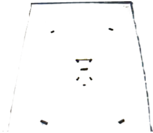
Figure 2: A convergence images captured by the CCD camera. As it can see the image distortion is increasing from bottom of image to top of image.
