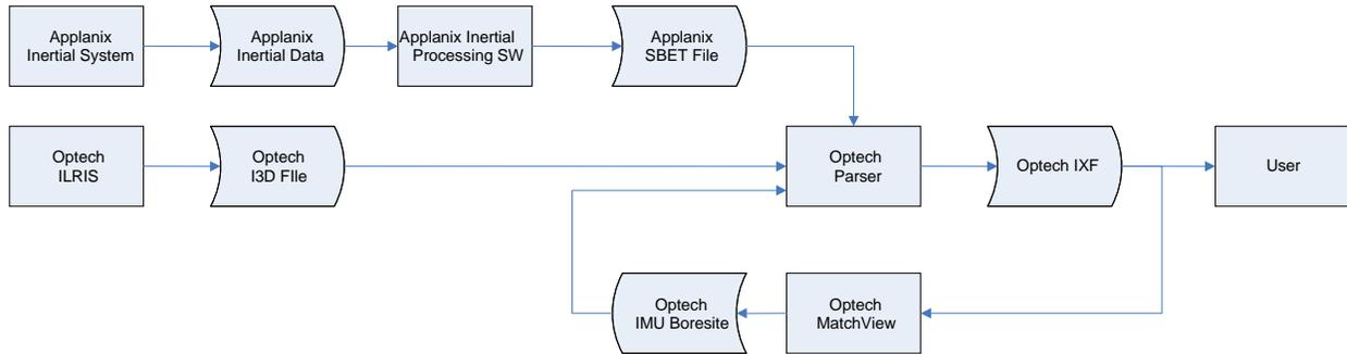
The resulting Optech IXF file contains a fully geo-referenced point cloud data set in WGS84 coordinates.
