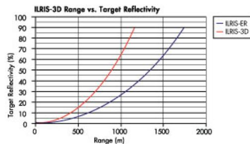
Figure 1: A comparison of range and target reflectivity, ILRIS-3D and ILRIS-ER.
