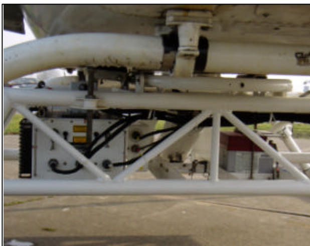
Figure 8. The sensor rack attached to an AS350 helicopter
