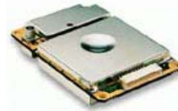
Figure 4. Garmin GPS25 sensor board
