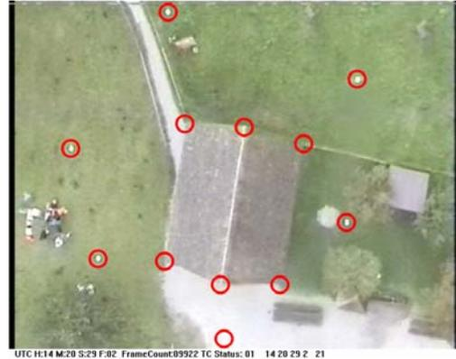
Figure 3: Test field for camera calibration
