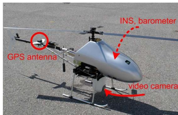
Figure 1: Mini UAV system Copter 1B (weControl / SurveyCopter)
