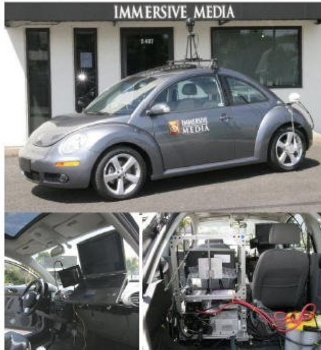
**Figure 5: Telemmersion® data collection vehicle with Applanix POS/LV 200 navigation system**
