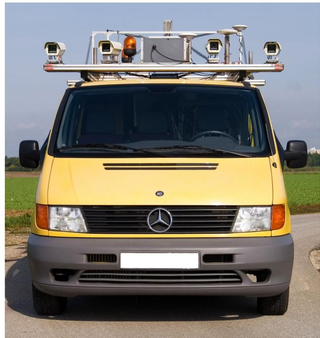
Figure 1. Mobile road Mapping System (MoSES).
