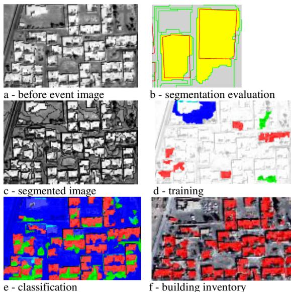
Figure 4. Flow diagram for building inventory.
