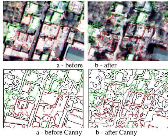
Figure 5. a) Before event image, b) after event image, c) Canny filtered before image, d) Canny filtered after image. In red, damaged buildings identified
