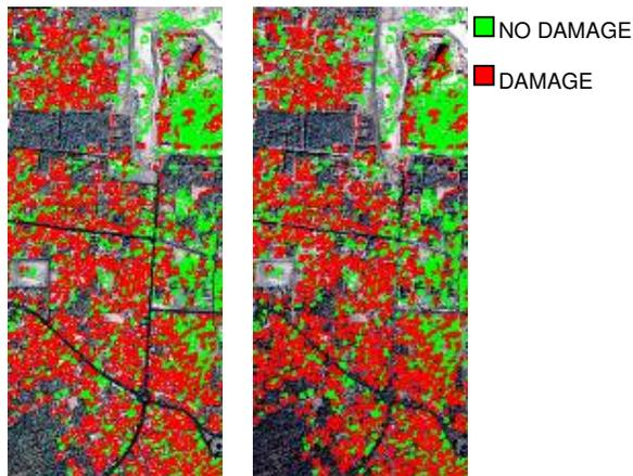
Figure 7. Results from change detection damage assessment. The before and the after event images are respectively in the left and in the right.
