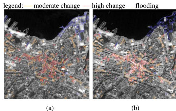
Figure 1. Before (a) and after (b) IRS images from Golcuk, overlaid with the damage assessment results.
