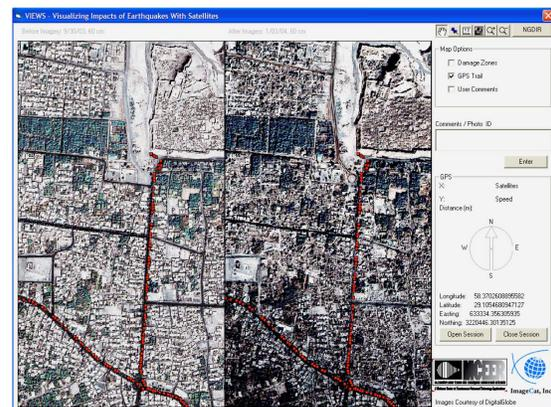
Figure 6. User interface of the VIEWS™ system used in Bam by the EERI reconnaissance team. GPS points are overlaid in the “before” and “after” satellite imagery, corresponding with routes driven through the city. GIS layers, such as texture based damage maps (Huyck et Al., 2005) can also be displayed.
