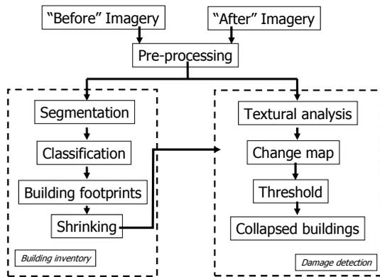
Figure 3. Damage detection from Quickbird imagery
