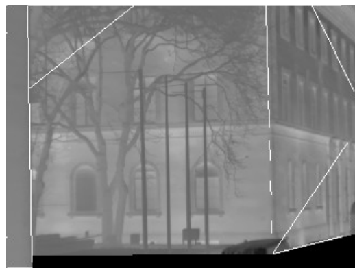
Figure 1. At first glance the polygons fit well, but the scale cannot be estimated because of missing vertices to correct the camera position
