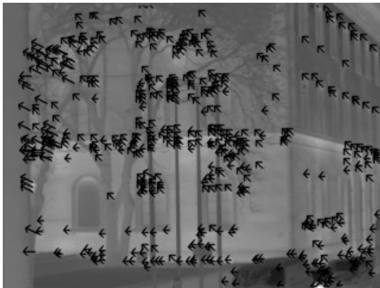
Figure 3. IR image with selected points of interest, that have correspondences in the following image. Arrows show the moving direction of the point
