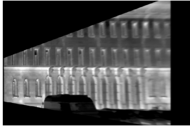
Figure 4. Partial texture of one façade extracted from the IR image in Figure 1 and Figure 2
