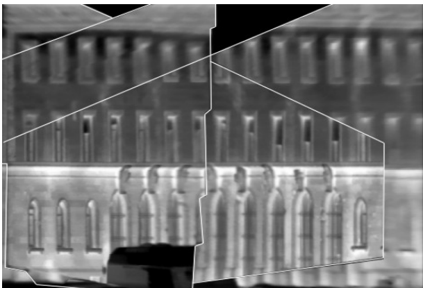
Figure 7. Surface texture generated from 3 partial textures. The edges between the taken textures are highlighted
