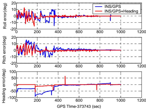
Figure 8: Attitude errors after utilizing heading sensor
