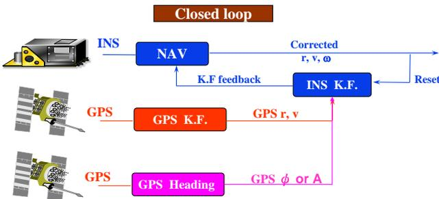
Figure 2: Modified INS/GPS integration scheme with GPS heading update
