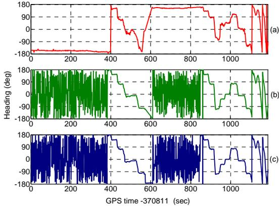
Figure 5: Three approaches to derive headings: (a) through the positional differences between two GPS antennas; (b) derived through the velocities of a GPS receiver; (c) using the displacement of a GPS antenna between two consecutive epochs
