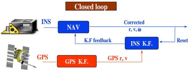
Figure 1: A standard INS/GPS loosely coupled integration scheme
