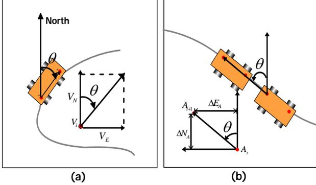
Figure 4: Computing heading from the velocities and position displacement
