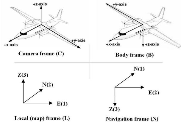
Figure 1: Coordinate systems used in navigation and photogrammetry.
