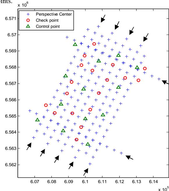
Figure 2. Perspective centers of the images of 1:5000 flight along with the control and check points. Arrows indicate the direction of the flights.
