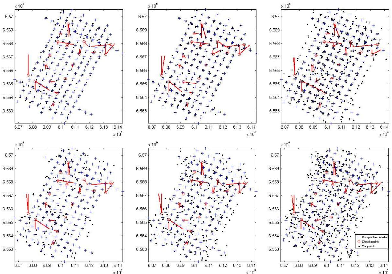
Figure 3. Vectors of error in check points obtained by using various tie point selection and distribution schemes in integrated orientation. Top row: regular distribution; bottom row: random distribution; from left to right: selection schemes S-1, S-2 and S-3.
