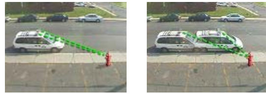
Figure 5. Stereoscropy using dual (left) and single (right) camera
