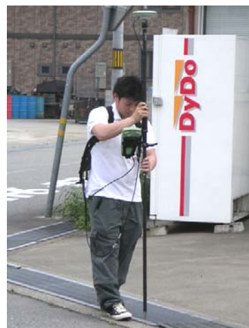
Figure 8. VRS-GPS on the road line
