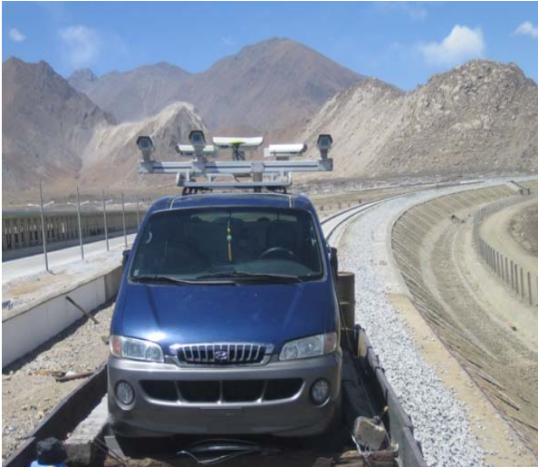
Figure 1 LD2000-RH MMS for Tibet Railway Surveying
