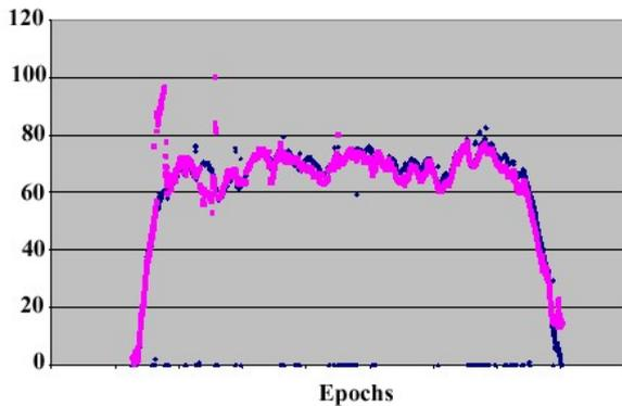
Figure 3 - Velocities (Km/h) computed from positions (blue) vs. velocities estimated by Doppler effect (magenta), for one of the test runs
