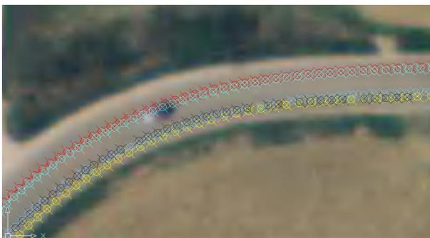
Figure 4 – GNSS kinematic survey to study the behaviour of a driver in relation with the road geometry
