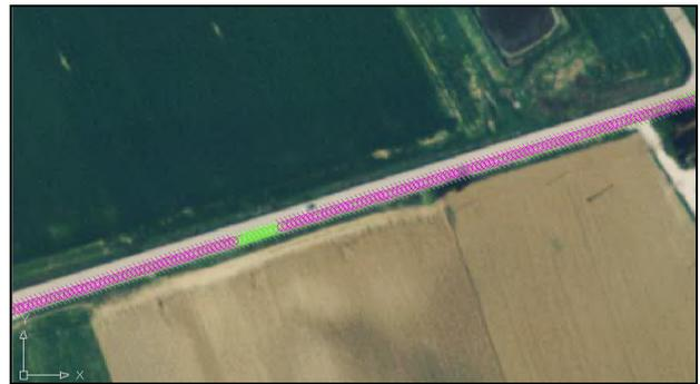
Figure 6a – Particular of the first part of the survey with good and converging solutions (Green: GNSS points; Magenta: IMU points)
