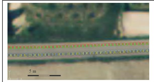
Figure 2 – Particular of some surveyed paths superimposed on a 1:10.000 orthophoto
