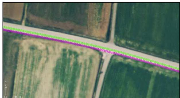
Figure 6c – Particular of a road stretch with no Omnistar correction and evident drift effect (the IMU solution in magenta colour falls out of the road)
