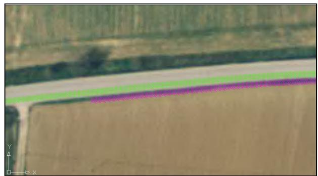
Figure 6b – Particular of a road stretch with no Omnistar correction and evident drift effect (the IMU solution in magenta colour falls out of the road)
