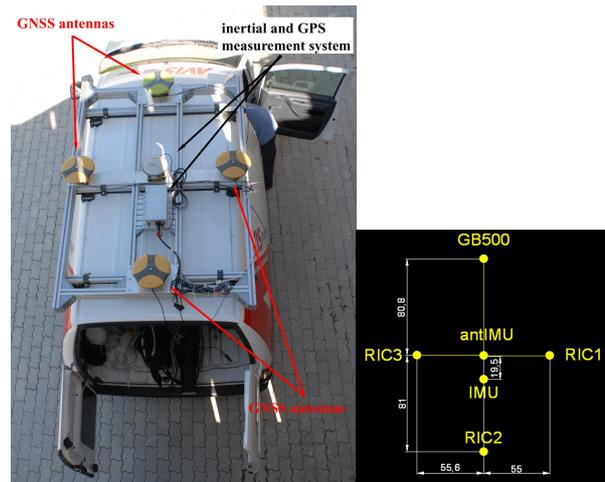
Figure 5 – MMV equipped for the tests and the instruments layout (measurements in cm)
