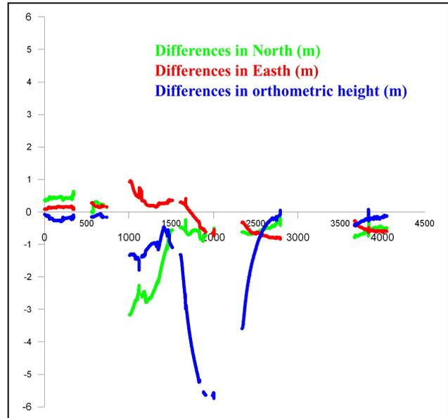
Figure 8 Graphs of position differences IMU vs GNSS
