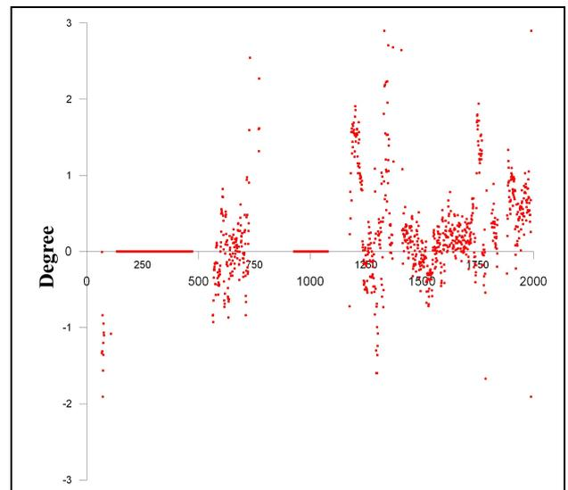
Figure 9 Heading differences between IMU and GNSS
