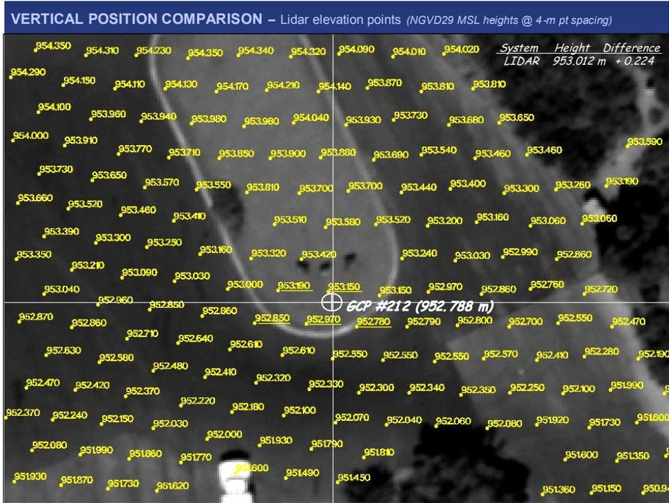
Figure3. Optical image vertical comparison with ALMS Lidar points
