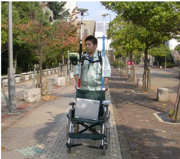
Figure 4. Positioning of D-GPS and VRS-GPS
