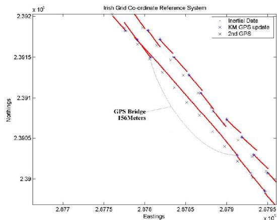
Figure 6. Primary GPS with satellite error (Road Section B)
