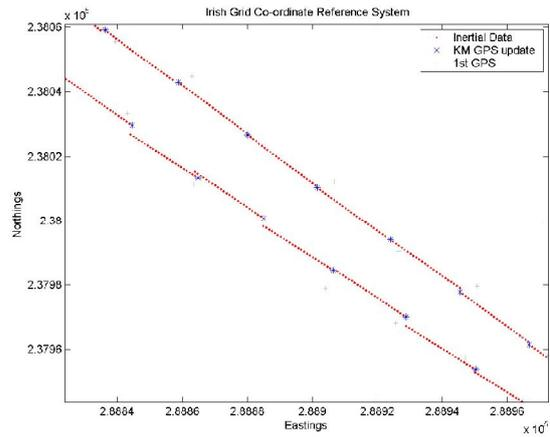
Figure 9. Section B EKF updates from second GPS receiver
