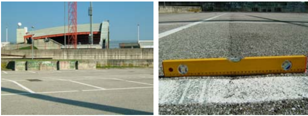
Figure 3. Left, the area of the test, only roughly horizontal; right, an irregularity of the asphaltting in elevation and in slope.
