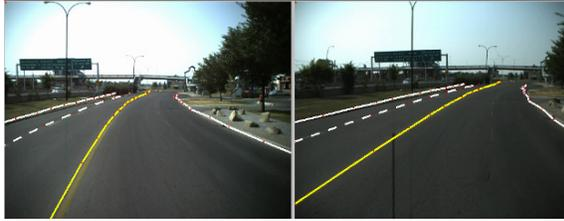
Figure 10: Example of miss detection to worn-out lane line
