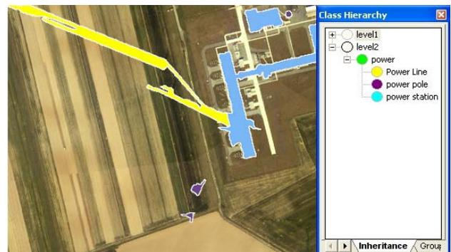
Figure 5. Extraction of power lines, power poles and power station in eCognition based on a LiDAR-DSM and spectral information from aerial photographs. Smaller power lines couldn't be extracted.
