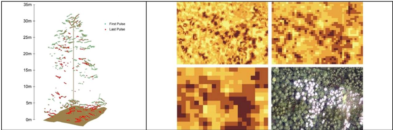
Figure 3. Left: 3d point cloud from both, first and last pulse data falling within the outline polygon of one identified tree. Right: Resulting height standard deviation based on moving windows at three different scales for a forest stand (lower right). Window sizes are 5m (upper left), 10m (upper right), 20m (lower left). Dark colours indicate higher values.
