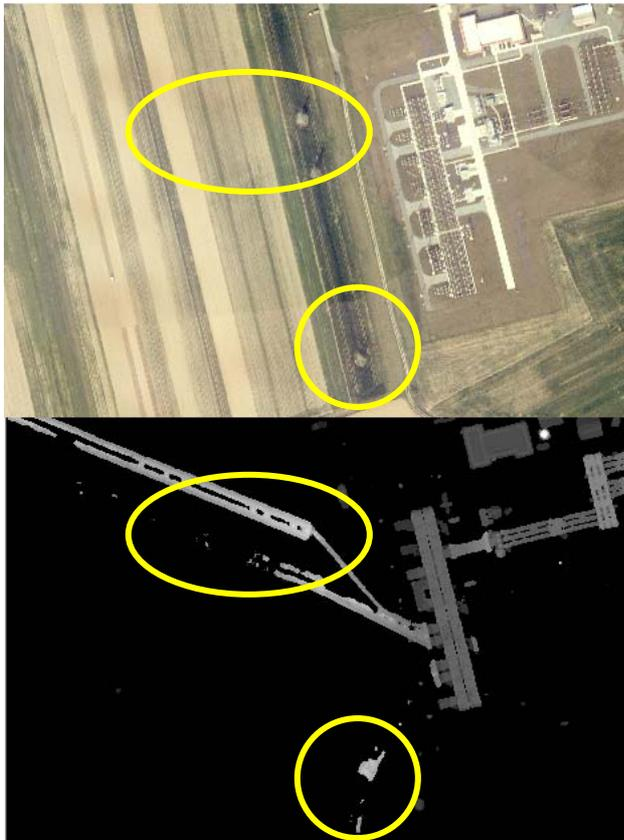
Figure 4. Aerial photograph (top): Power lines not visible, power poles visible. LiDAR DSM (bottom): Bigger power lines and power poles visible, smaller power lines intermittent visible.
