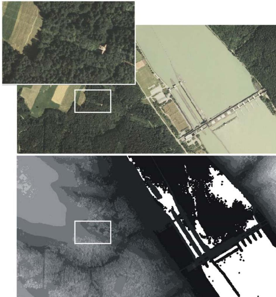
Figure 7. RGB aerial photographs (top): Power lines visible (see zoom window). LiDAR data (bottom): Pulse density too coarse to detect power lines.
