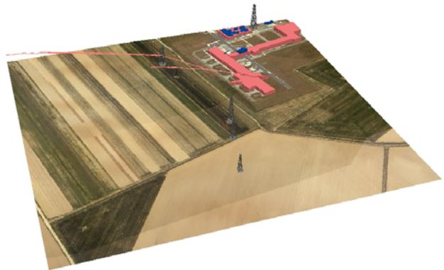
Figure 6. 3D Visualization of extracted objects extruded by LiDAR height information.
