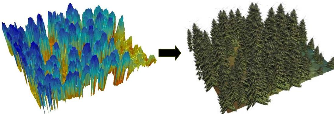
Figure 2. Extraction and visualization of trees from a LiDAR derived DSM and multi-spectral information.
