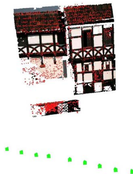
Figure 8. Frontal view, seen slightly from above of the same scene as in Fig. 7. On the lower side the green pyramids show the estimated positions of the cameras. For the wall in front of the building, the parts which have a pattern of holes can be distinguished from the solid parts.
