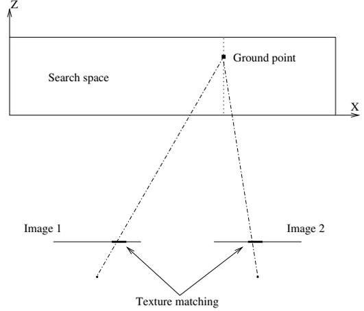
Figure 3: Reprojection of a ground point in the images. Top view.
