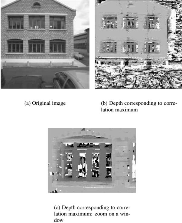
Figure 7: Image-space depth extraction. Correlation window size: 3 pixels, depth pitch: 2cm.
