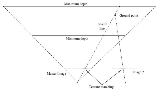
Figure 6: Search line from a given pixel in the master image. Reprojection of a ground point hypothesis in the other images. Top view.
