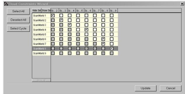
Figure 5: Matrix-based scheme for the pairwise registration
