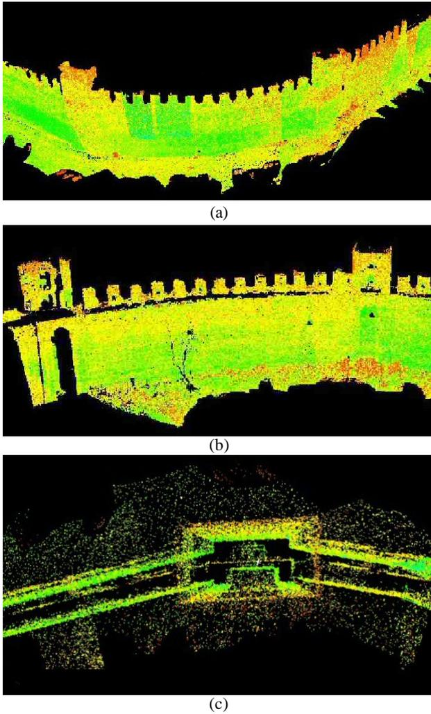
Figure 7: Views of the aligned scans of the outside (a) and inside walls (b); unified global model (c)
