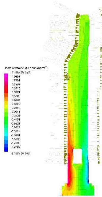
Figure 9: Color map showing the effect of the vertical stresses due to the wind
