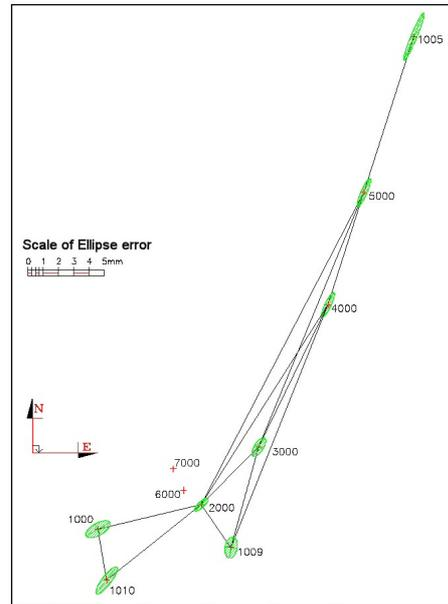
Figure 2: The local network surveyed with the total station
