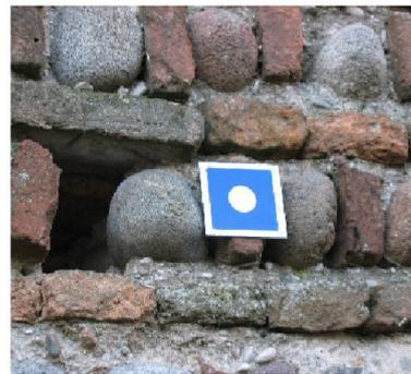
Figure 3: Example of retroreflective target used for laser scan registration and georeferencing
