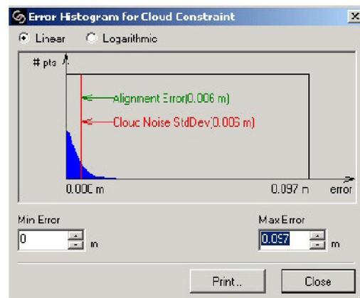
Figure 6: Example of the RMS of a pairwise registration
