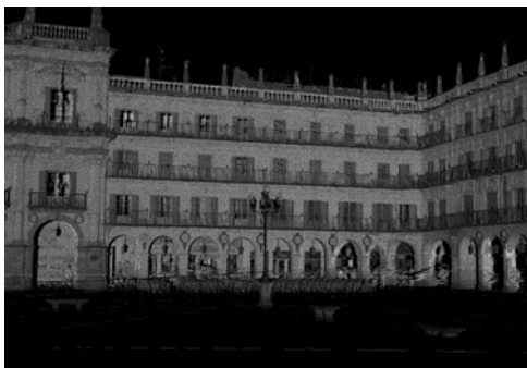
Figure 10: An smart adaptive optimised reduction of the original cloud of points for the Plaza Mayor of Salamanca
