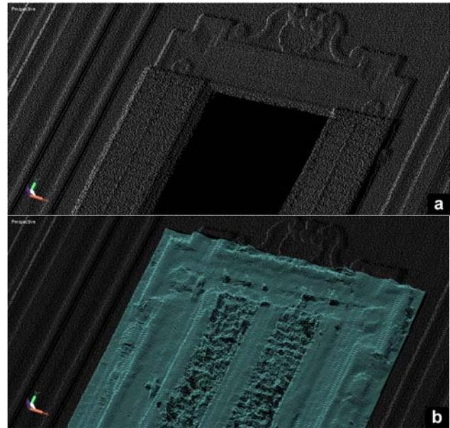
Figure 9. Area of the right window: a) laser scanner point cloud, b) integration with photogrammetric points
