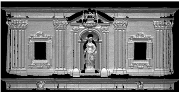
Figure 6. Triangulated surface extracted from laser data
