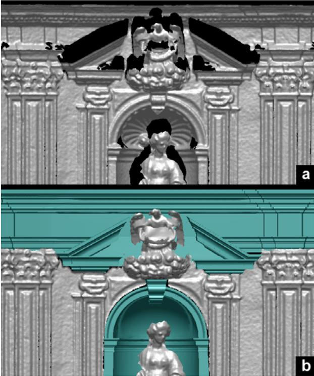
Figure 10. Area of the tympanum: a) triangulated surface from laser scanning data, b) integration with CAD models
