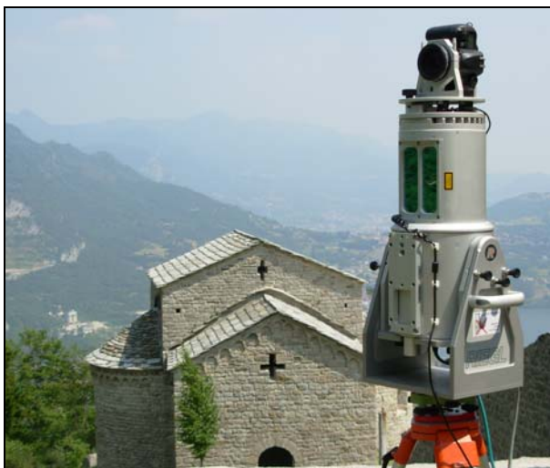
Figure 4: laser scanner RiegI LMS-Z420i with its integrated camera during scanning of the oratorio di San Benedetto roof.
