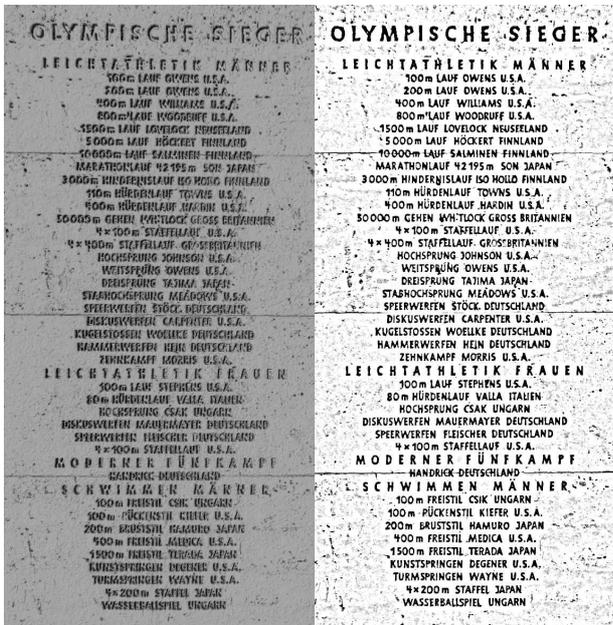
Figure 9: Two representations of a 3D model build from photogrammetry and shape from shading. Left: regular shading, Right: relative depth analysis and histogram adjustments.
