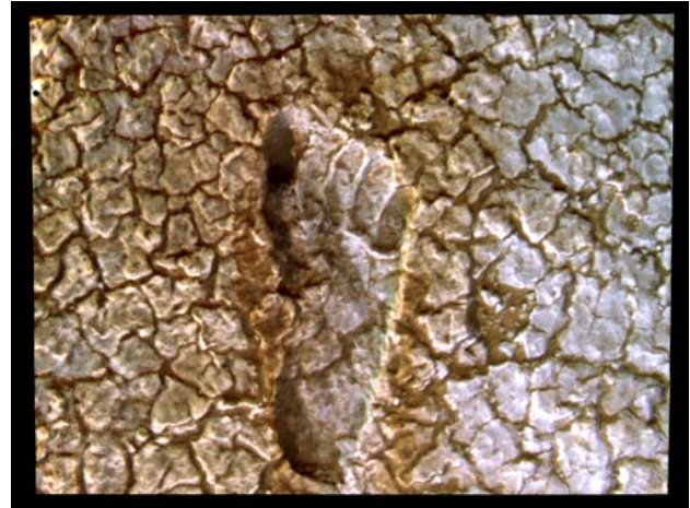
Figure 9: Image of rendered laser scan data of a fossilised human footprint with solar illumination. Data acquired with a KonicaMinolta Vivid 910. Image © The University of Melbourne
