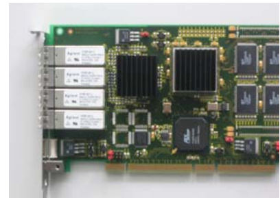
Figure 6 LLPC Electronics Components AD-Board, Interface-board und 64Bit Frame-Grabber
