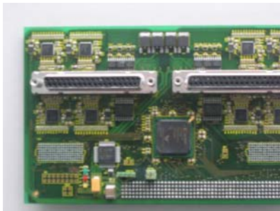
Figure 6 LLPC Electronics Components AD-Board, Interface-board und 64Bit Frame-Grabber
