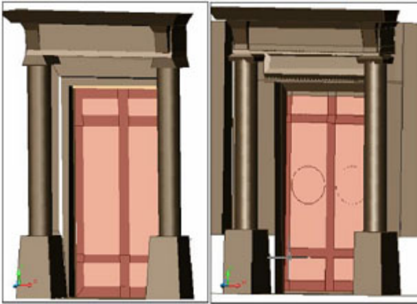
Fig. 6: Level of detail of the 3D model of one door in Großer Festsaal, constructed in the point cloud of GS100 (left) and IMAGER 5003 (right)
