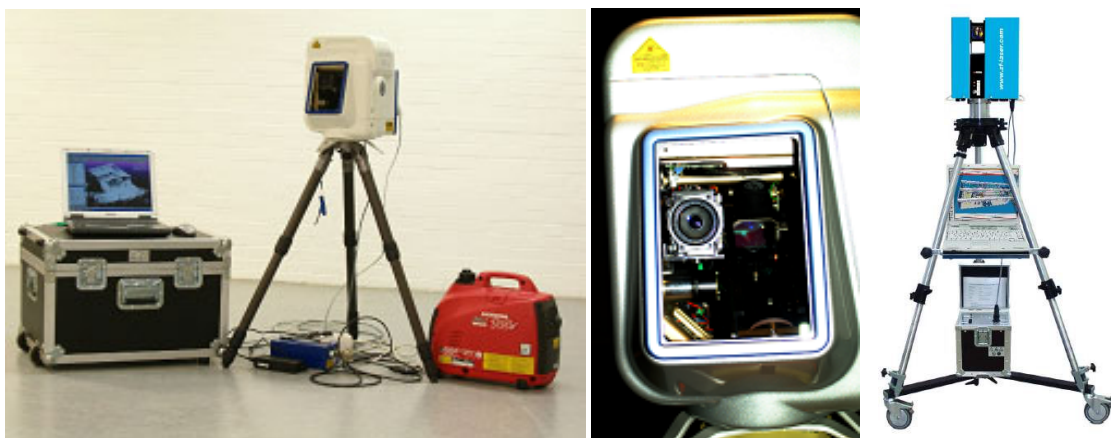
Fig. 2: The 3D laser scanning system Mensi GS100 of HAW Hamburg with accessories (left), GS100-interior with digital camera and mirror (middle), IMAGER 5003 with accessories (right)
