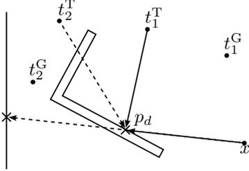
Fig. 9: Occlusions in texture images have to be considered in the weighting process. The texture at  $t_2^T$  may not contribute to the color of point  $p_d$ , since it is occluded.
