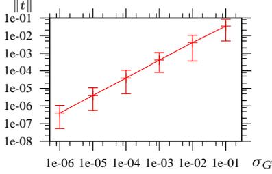
Fig. 8: Shown is the error  $\|t\|$  of the final estimation for  $t$  depending on the noise in  $L_i^G$ . Displayed is the average, minimum, and maximum of 100 test-runs.
