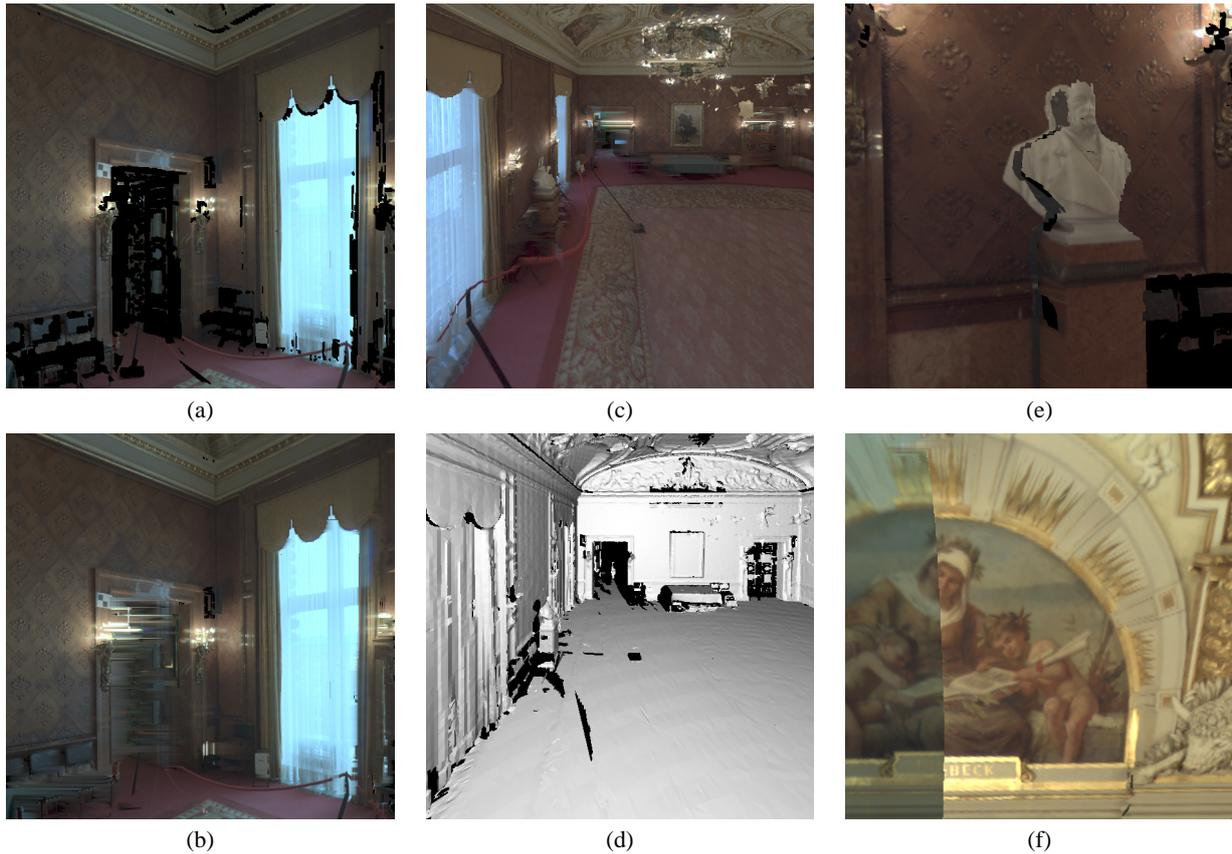
Fig. 11: The most obvious quality problems in the background shots are: missing geometry and texture information (a, b); overlooked geometry (c, d); and insufficient texture registration precision (e, f).
