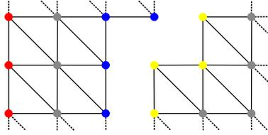
Fig. 5: Adjacent points in the depth image are connected to form a triangle mesh. Points from different surface patches are not connected. Red dots belong to class *verge*, blue to *back edge*, yellow to *front edge*, and grey to *surface*.
