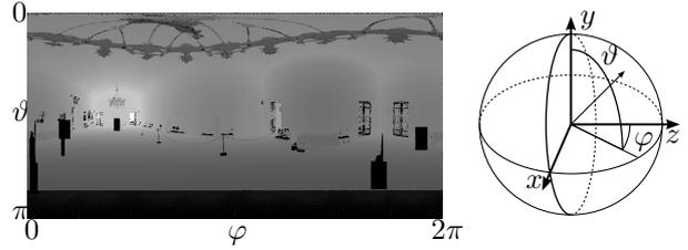
Fig. 3: Full spherical depth image with its parameterization and its associated local left hand coordinate system. The brighter the image pixel is, the further away is the respective object. The displayed range is approximately 1m to 25m.
