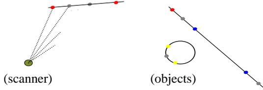
Fig. 4: Shown is a schematic 1D example scan including points of each class. Red dots belong to class *verge*, blue to *back edge*, yellow to *front edge*, and grey to *surface*.
