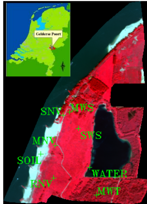
Figure 1. HyMap image for the Millingerwaard floodplain along the river Waal. The indicated points show the location of 'pure' PFTs from the field polygons for which spectral endmembers were derived from the image. Inset shows the location of the floodplain within the Gelderse Poort nature reserve.
