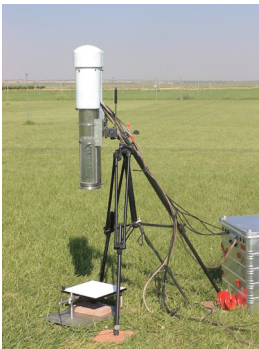
Figure 1. TerFlex sensor in its measuring configuration.
