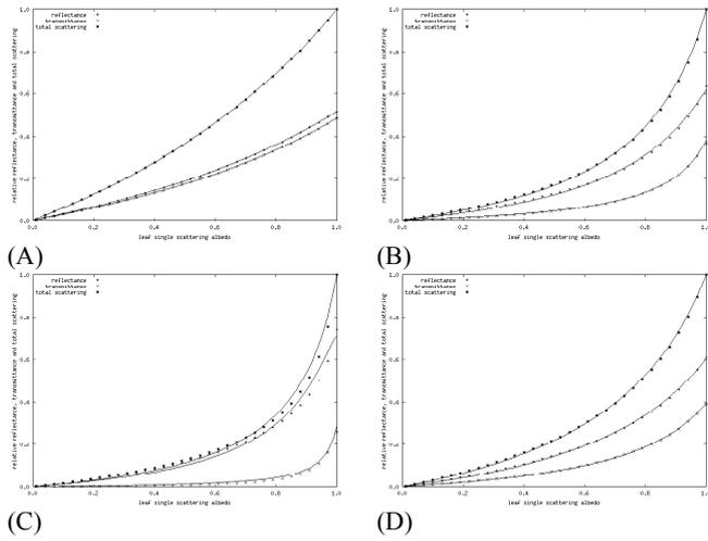
Figure 3a. Relative reflectance, transmittance and total scattering as a function of leaf single scattering albedo, for the canopies (A,B,C,D) for  $\zeta=0.5$ , zenith  $0^\circ$  (symbols), with lines showing fitting of the original model.
