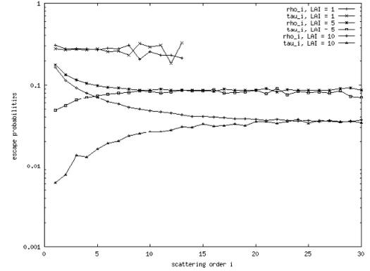
Figure 2. Upward and downward escape probabilities as a function of scattering order for homogeneous canopies at LAI 1, 5 and 10,  $\zeta = 0.5$ , zenith angle  $0^\circ$ .
