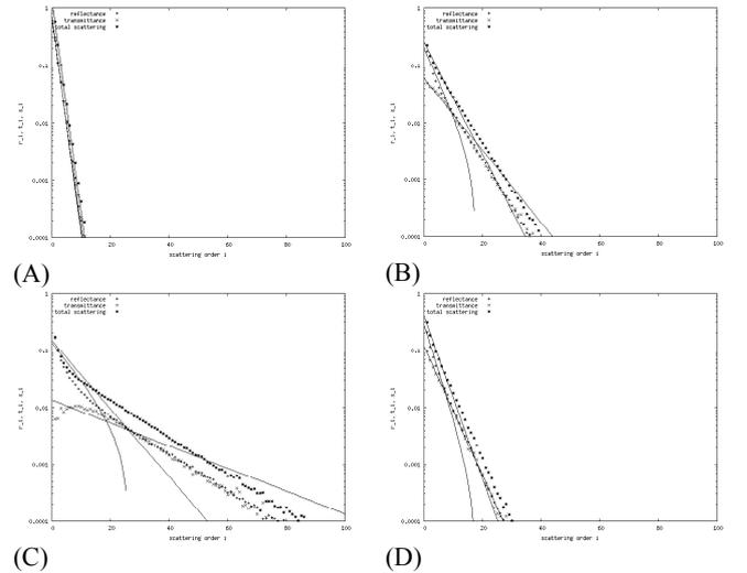
Figure 3c. Spectrally-invariant terms as a function of scattering order for canopies A, B, C and D for  $\zeta=0.5$ , zenith  $0^\circ$  (symbols), with lines showing the original model.
