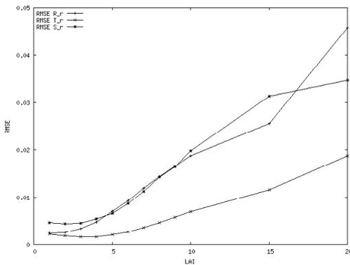
Figure 3b. Root mean square error (RMSE) for relative reflectance, transmittance and total scattering for the homogeneous canopies as a function of LAI.
